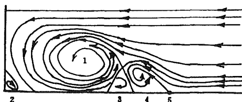
Fig. 3(b) Flow model near leading edge: (1) horseshoe vortices; (2) corner vortices; (3) countervortices; (4) separation vortices; (5) separation points
